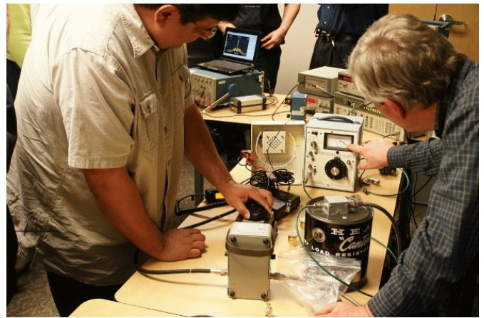
Gregg KF6FNA and Gary WB6YRU checking FM deviation
